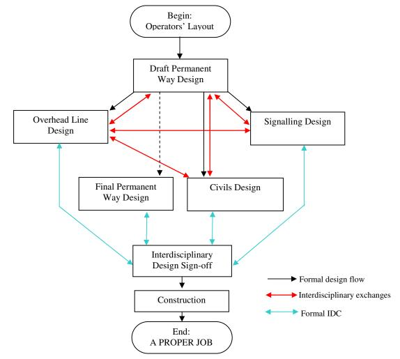
In this approach, the permanent way design takes the lead, albeit in draft, as it is best to have something to discuss first. The permanent way tend to do huge and detailed topographical surveys, allowing the other designers to verify locations of key features using real distances (rather that the arbitrary miles/kilometres/chains/yards/feet/links systems, none of which agree with the others).
